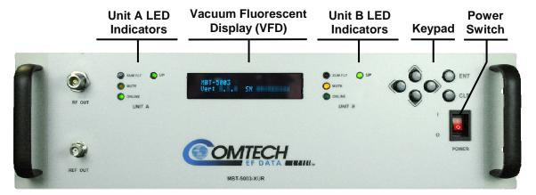
Figure 5-1. MBT-5003 Front Panel (MBT-5003-XUR shown)
