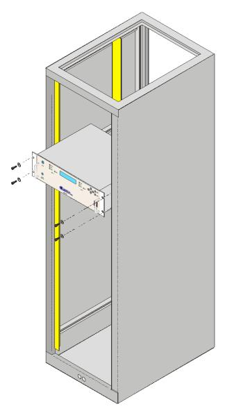
Figure 2-1. Standard Rack Cabinet Installation
